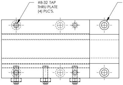
MTG. HOLE FOR #8 S.H.C.S. (6) PLC'S.
