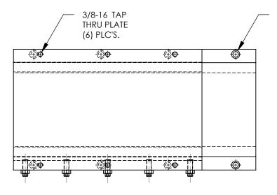
MTG. HOLE FOR 3/8 S.H.C.S. (8) PLC'S.
